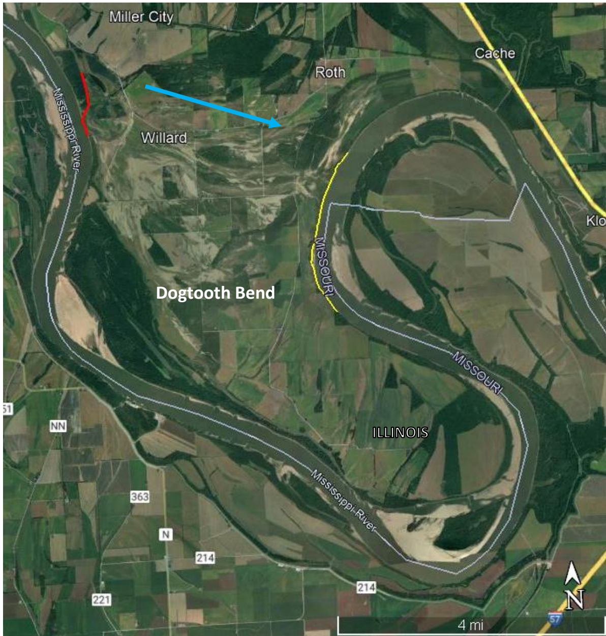
Figure 2. Water flow potential (blue arrow) to cut off channel from Len Small Levee breach (red line) to Dogtooth Bend proposed project area (yellow line), resulting in 17 miles reduced to 3.5 miles.
