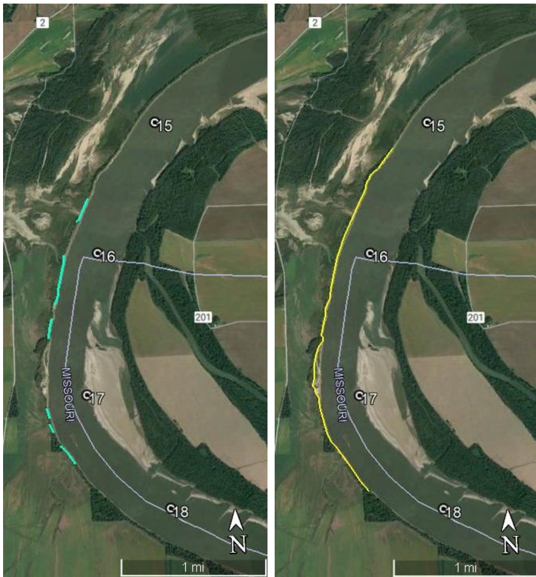
Figure 3. Proposed locations for landside (green) and riverside (yellow) bankline revetment within the proposed project area on Dogtooth Bend, Alexander County, Illinois.
