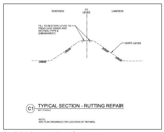
Figure 8. Typical cross section diagram of rutting repair.
