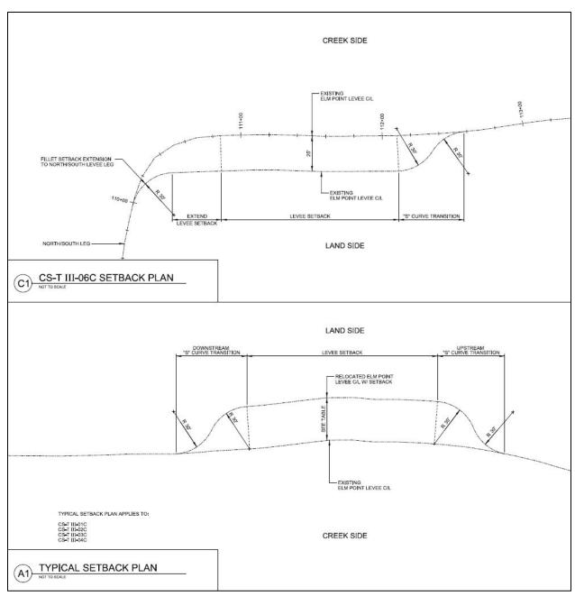
Figure 6. Proposed levee setback alignment.
