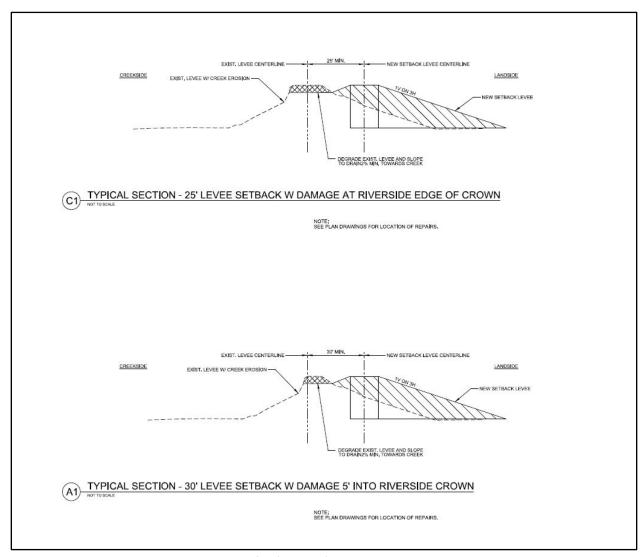
**Figure 5.** Typical cross section diagram of 25' and 30' levee setback.
