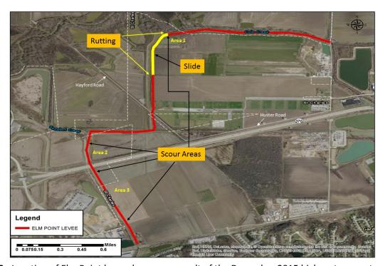
**Figure 2.** Location of Elm Point levee damage as result of the December 2015 high water event.
