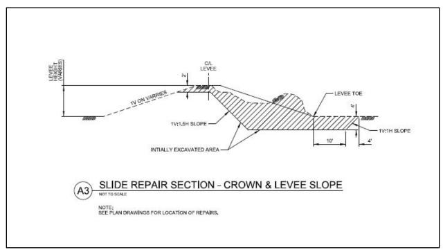
Figure 7. Typical cross section diagram of slide repair.
