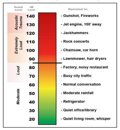
Figure 2. Examples of the sound level and decibel (dB) level of various sources.
