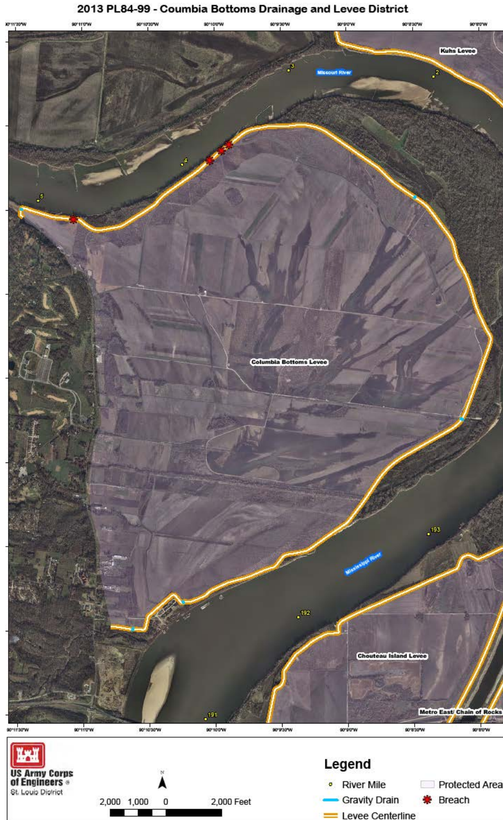
Figure 1 - Columbia Bottom Levee District and 2013 damages (four breaches).
