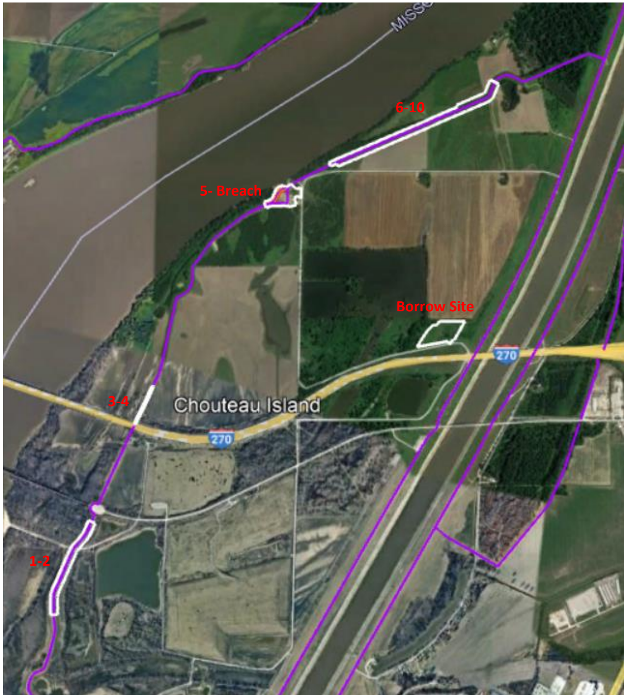
Figure 11. Extent of construction footprint shown outlined in white for all damage and borrow areas.
