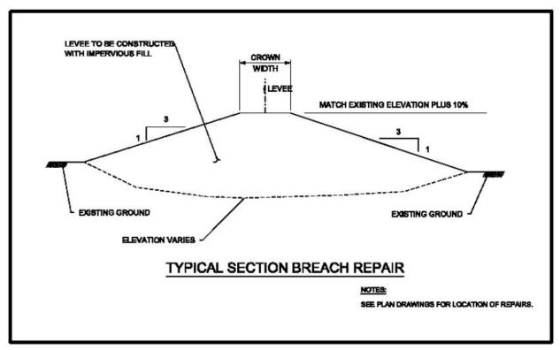
Figure 5: Proposed section/structural repairs for breaches.
