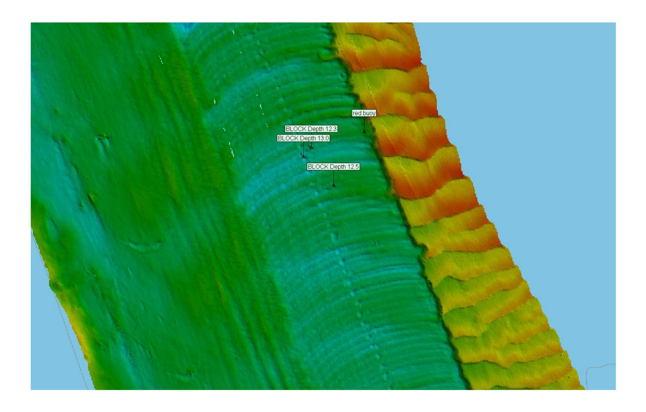
Possible buoy rocks located from 60-ft to 80-ft left of sailing line shown on IENC. Depths shown are actual depth at time of the survey. Valley City gage was 1.25-ft above minimum pool. Subtract 1.25-ft to get depth at minimum pool. Block Depth = 12.3 -1.25 = 11.0-ft at minimum pool. Block Depth 12.5 -1.25 = 11.2-ft at minimum pool. Block Depth 13.-0 - 1.25 = 11.7-ft at minimum pool.
