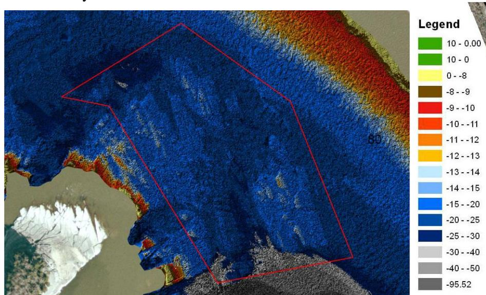
Figure 4: Work Area GT2P is located at approximately River Mile 79.0. This work area consists of hard, dense limestone shelf rock. All material above an elevation of 309.7 ft NGVD 1929 (-13 ft design plane) is to be removed. The estimated quantity of material to be removed is 562 cubic yards.
