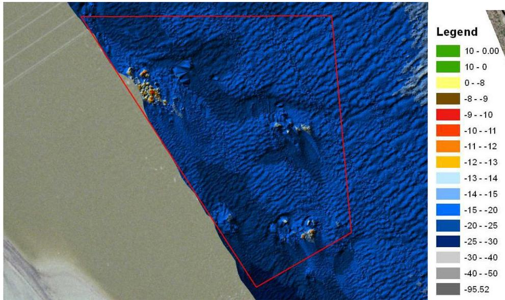
Figure 16: Work Area TR11P is located at approximately 38.5. This work area consists of limestone pinnacle rock. All material above an elevation of 287.7 ft NGVD 1929 (-13 ft design plane) is to be removed. The estimated quantity of material to be removed is 1776 cubic yards.
