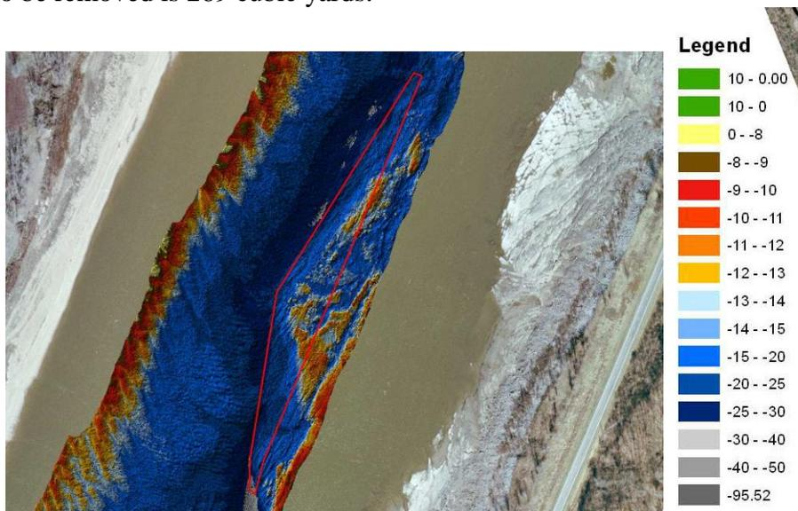
Figure 9: Work Area TR4P is located at approximately River Mile 44.5. This work Area consists of limestone pinnacle rock. All material above an elevation of 291.3 ft NGVD 1929 (-13 ft design plane) is to be removed. The estimated quantity of material to be removed is 663 cubic yards.
