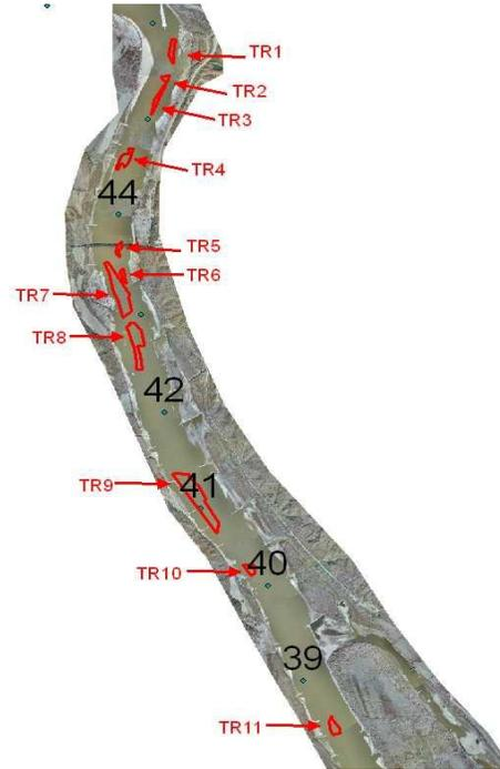
Figure 6: Work Area TR1P is located at approximately River Mile 45.7. This work area consists of limestone pinnacle rock. All material above an elevation of 291.9 ft NGVD 1929 (-13 ft design plane) is to be removed. The estimated quantity of material to be removed is 54 cubic yards.
