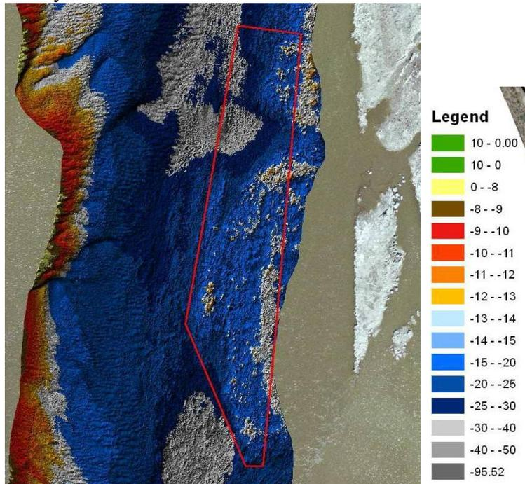
Figure 7: Work Area TR2P is located at approximately River Mile 45.5. This work area consists of both limestone shelf rock and pinnacle rock. All material above an elevation of 291.7 ft NGVD 1929 (-13 ft design plane) is to be removed. The estimated quantity of material to be removed is 457 cubic yards.
