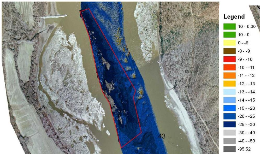
Figure 13: Work Area TR8P is located at approximately River Mile 42.8. This work area consists of both limestone shelf rock and pinnacle rock. All material above an elevation of 290.1 ft NGVD 1929 (-13 ft design plane) is to be removed. The estimated quantity of material to be removed is 187 cubic yards.
