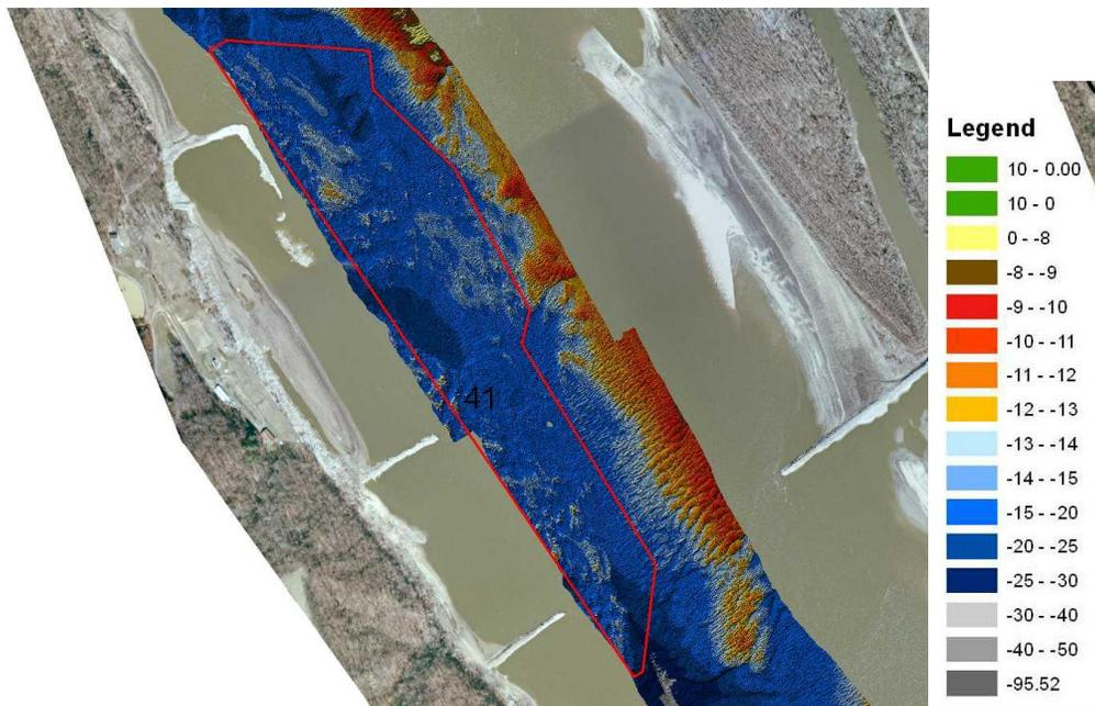
Figure 15: Work Area TR10P is located at approximately River Mile 40.2. This work area consists of limestone pinnacle rock. All material above an elevation of 288.4 ft NGVD 1929 (-13 ft design plane) is to be removed. The estimated quantity of material to be removed is 28 cubic yards.
