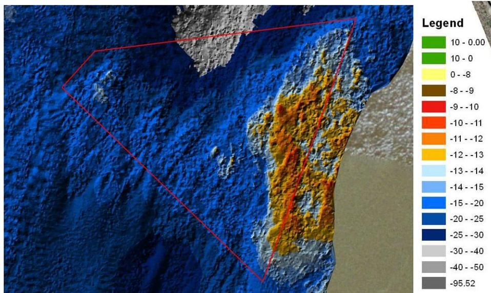
Figure 8: Work Area TR3P is located at approximately River Mile 45.2. This work area consists of both limestone shelf rock and pinnacle rock. All material above an elevation of 291.6 ft NGVD 1929 (-13 ft design plane) is to be removed. The estimated quantity of material to be removed is 269 cubic yards.
