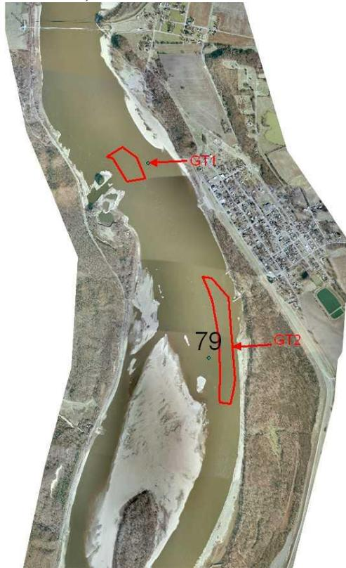
Figure 3: Work Area GT1P is located at approximately River Mile 80.0. This work area consists of limestone pinnacle rock. All material above an elevation of 311.5 ft NGVD 1929 (-13 ft design plane) is to be removed. The estimated quantity of material to be removed is 2 cubic yards.
