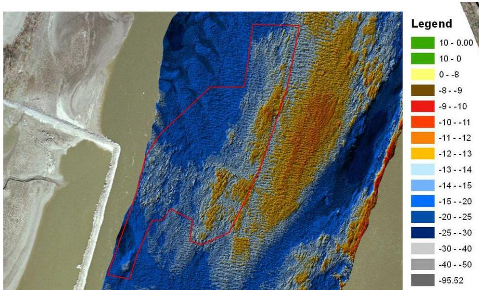
Figure 10: Work Area TR5P is located at approximately River Mile 43.5. This work area consists of limestone pinnacle rock. All material above an elevation of 290.8 ft NGVD 1929 (-13 ft design plane) is to be removed. The estimated quantity of material to be removed is 327 cubic yards.
