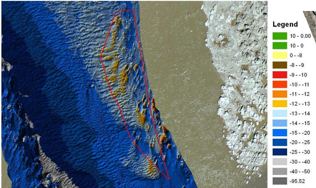
Figure 12: Work Area TR7P is located at approximately River Mile 43.2. This work area consists of limestone pinnacle rock. All material above an elevation of 290.3 ft NGVD 1929 (-13 ft design plane) is to be removed. The estimated quantity of material to be removed is 32 cubic yards.
