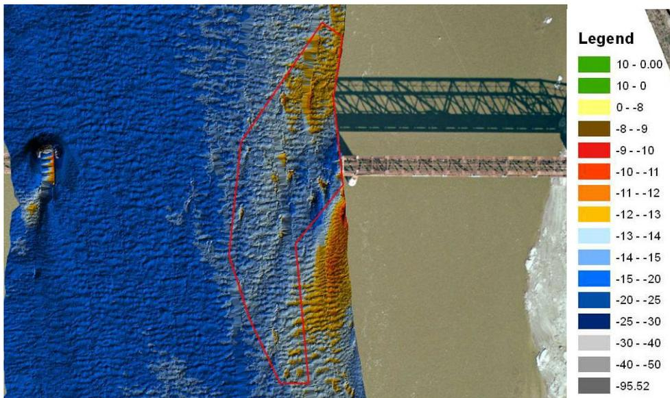
Figure 11: Work Area TR6P is located at approximately River Mile 43.4. This work area consists of limestone pinnacle rock. All material above an elevation of 290.3 ft NGVD 1929 (-13 ft design plane) is to be removed. The estimated quantity of material to be removed is 183 cubic yards.
