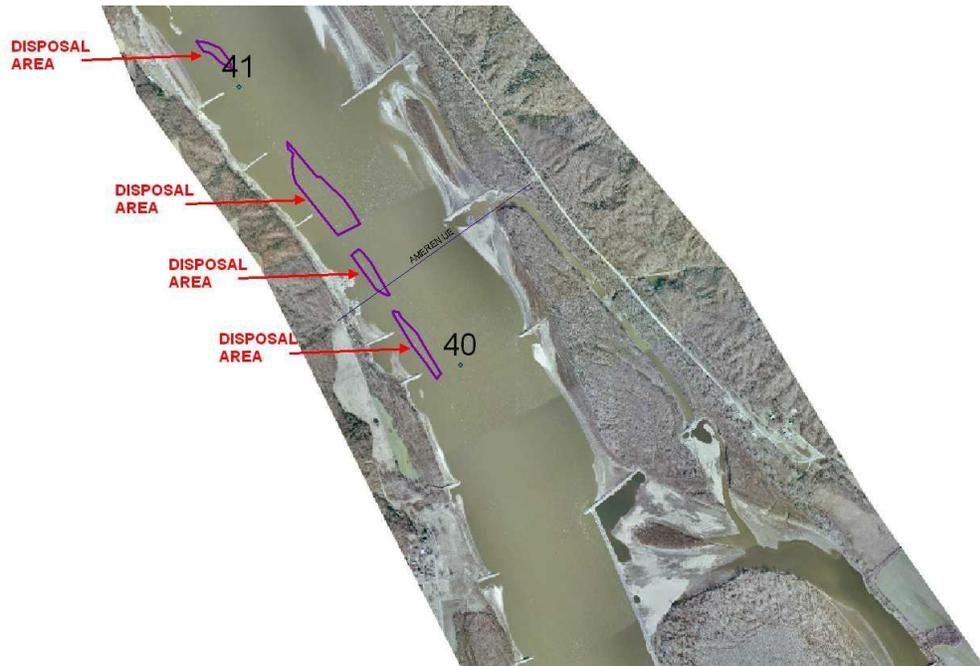
Figure 18: Disposal area for material excavated from the channel area adjacent to Cottonwood Island (Thebes Gap Reach). The material is to be used to create a gravel/rubble area at the head of an existing bar.
