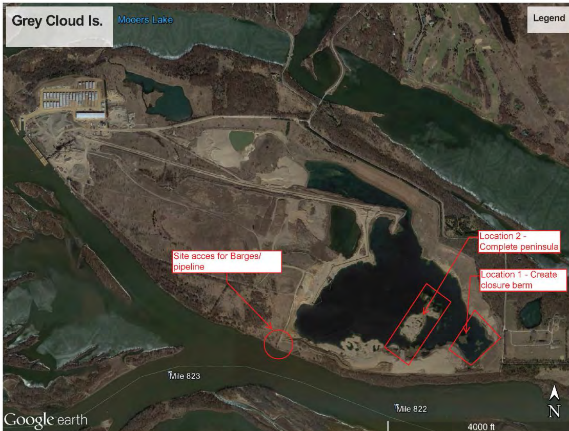
Figure 5-3 Proposed Dredged Material Placement Site for Alternative 6
