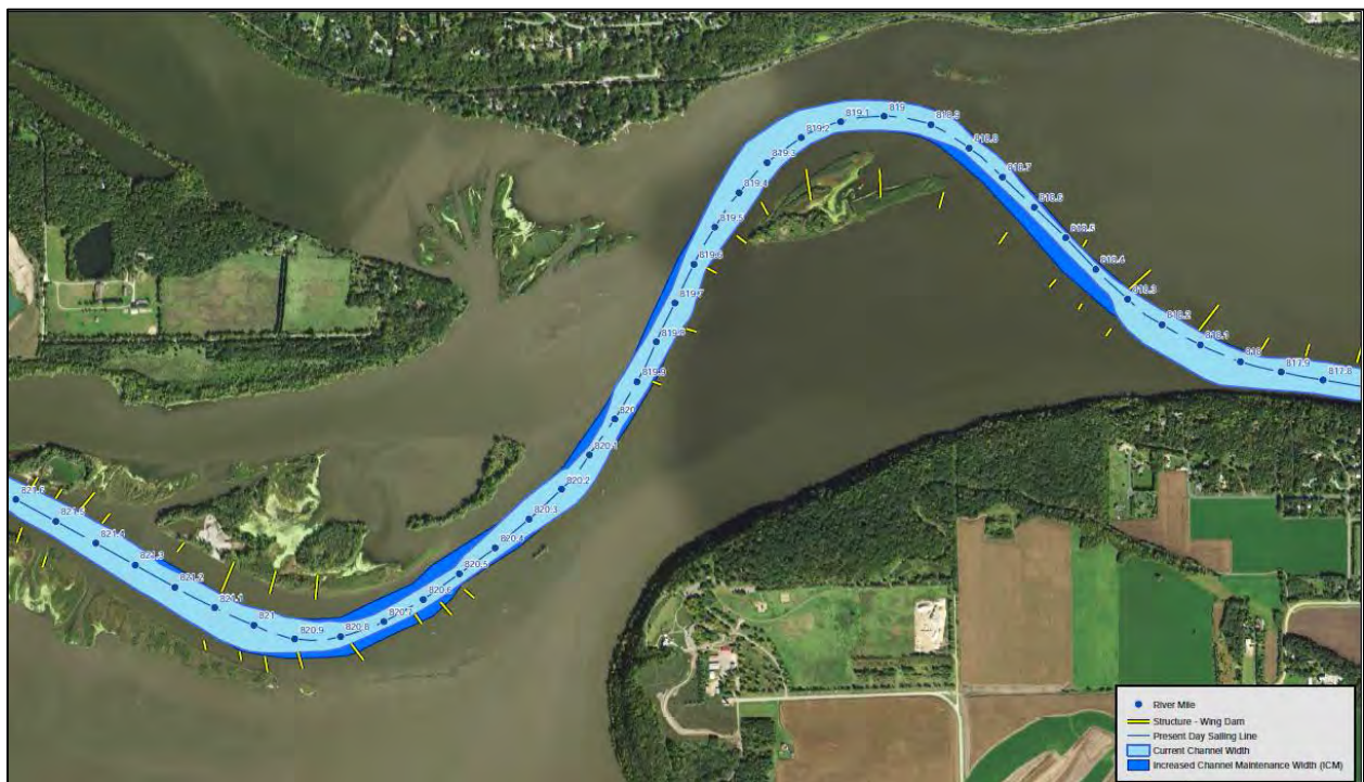
Figure 4-3 Increased Channel Maintenance Corridor and Current Width Comparison
