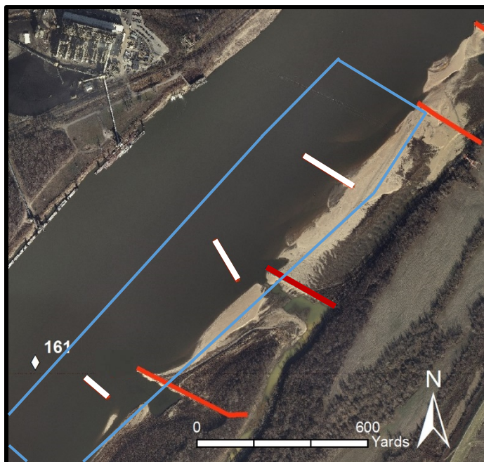
Figure 11. 2012 Aerial imagery of the Mosenthein-Ivory Landing Phase 5 work area, including the new rootless dike structures (white), existing river training structures (red), and total area of influence (blue).
