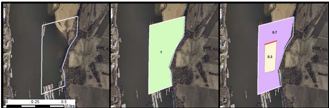
Figure 4. Delineation of the total area of influence (left) as well as pre- (center) and post-construction (right) delineation of the structured/unstructured parameter categories for the Mosenthein Ivory Landing Phase 4 work area. Construction of the rootless dike (red) reduces the score immediately downstream of the dike to 0.3, and the remainder of the area to 0.7, because a dike is now present within the total area of influence.
