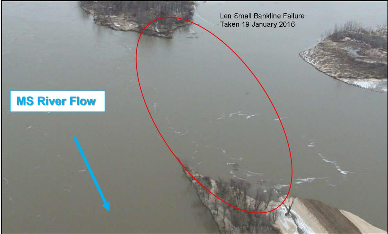
Figure 3. Bankline failure during January 2016
