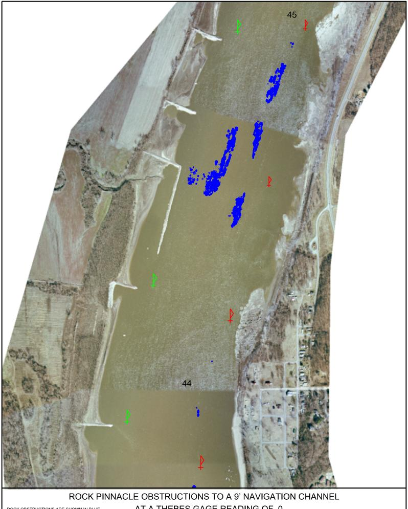
ROCK OBSTRUCTIONS ARE SHOWN IN BLUE 2006 ROCK PINNACLE SURVEY 2006 AERIAL PHOTO BUOY LOCATIONS ON APRIL 12,2012. THEBES GAGE 15.5 AT A THEBES GAGE READING OF 0
