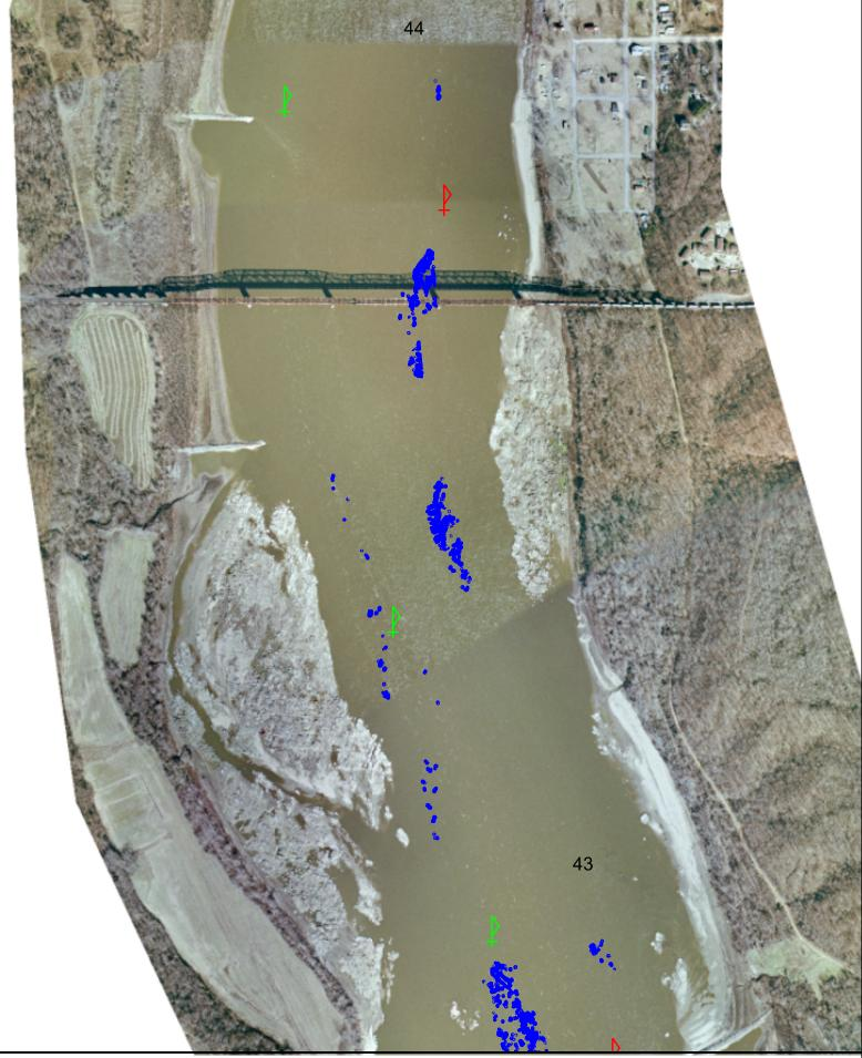
ROCK PINNACLE OBSTRUCTIONS TO A 9' NAVIGATION CHANNEL ROCK OBSTRUCTIONS ARE SHOWN IN BLUE AT A THEBES GAGE READING OF 0
