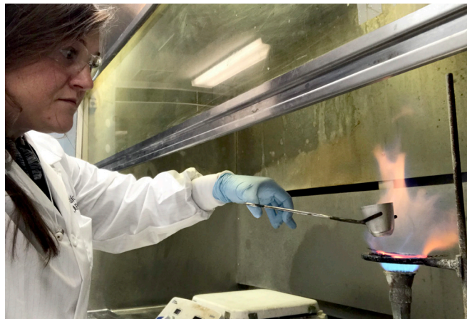
A specially trained laboratory chemist separates thorium from other isotopes in a sample so thorium alone can be measured by alpha spectroscopy.
