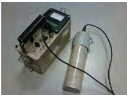
Ludlum 2221 (scaler, ratemeter) with 44-10 probe (2"x 2", NaI Scintillator)
