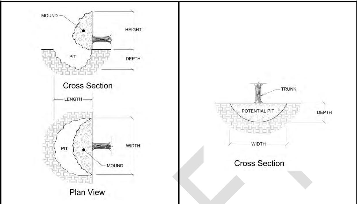
**a. Assumed Pit/Mound** (above). The *assumed pit/mound* represents the typical configuration and maximum likely dimensions of an overturning alteration to the cross section. It is provided as a standard basis for scour analysis.
