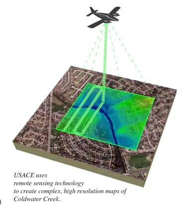
three-dimensional data about the earth's surface. GIS specialists produce complex, high resolution maps called digital elevation models using LIDAR data. These models give USACE an understanding of the contour of CWC's floodplain and its surroundings.
